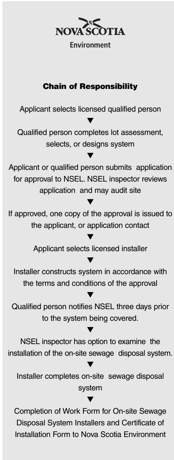
Figure 4 Approval Procedure Flowchart for an On-site System
